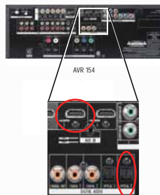
Figure 23 – Connecting an HDMI-Equipped Recorder
