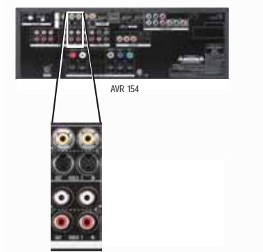
Figure 25 – Connecting a Video Recorder
