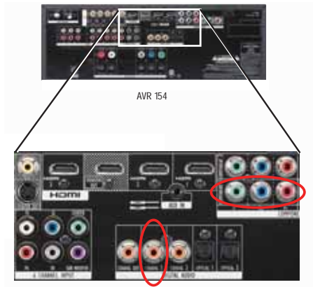
Figure 21 – Connecting a Component-Video-Equipped Disc Player
