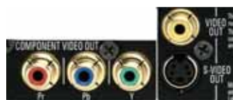
Figure 10 – Component, S- and Composite Video Outputs
