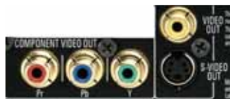
Figure 10 (repeated) – Component, S- and Composite Video Outputs
