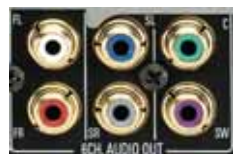
Figure 13 – 6-Channel Analog Audio Outputs
