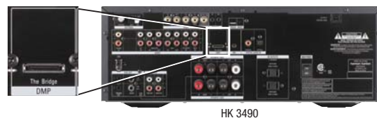
Figure 20 – The Bridge II Connection
