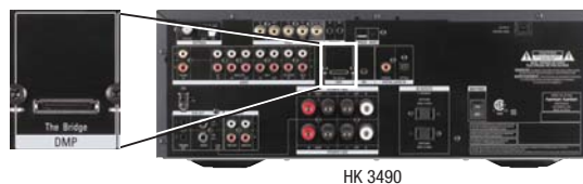
Figure 20 – The Bridge II Connection
