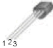
78L05, Voltage Regulator, TO-92
