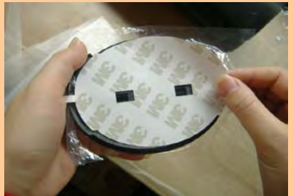
14 attach the side end cap ( peel off adhesive ) and add super glue
