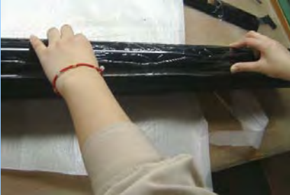
14 attach the side end cap ( peel off adhesive ) and add super glue
