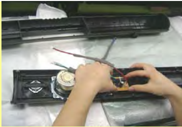
6 Plug green/black cables to the woofer, green cable for + polarity, and black for - polarity
