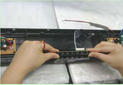
Screw down amp ( Screw X 9 pcs PN: 352-AM03008C1086-E )
