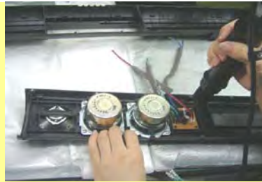
6 Plug green/black cables to the woofer, green cable for + polarity, and black for - polarity
