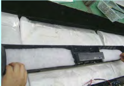
10 plug in xover harness to the amp
