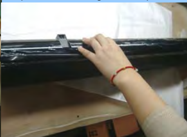
14 attach the side end cap ( peel off adhesive ) and add super glue
