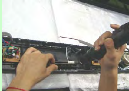
Screw down amp ( Screw X 9 pcs PN: 352-AM03008C1086-E )
