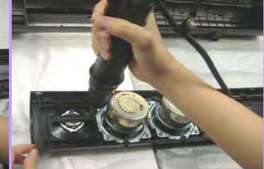
attach tweeter bar and screw down screw pn 352-AM03008C1086-E
