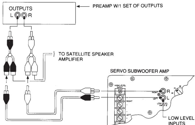
When using a single subwoofer, you must use a stereo pair of low-level leads from your preamp's outputs. When using two subwoofers, one for each channel, connect the left channel preamp out to both the Left and Right Low Level Input jacks of the subwoofer on the left by using a "Y" connector at the subwoofer's amplifier, and the right channel preamp out to both jacks of the subwoofer on the right in the same manner. See figure 5.
