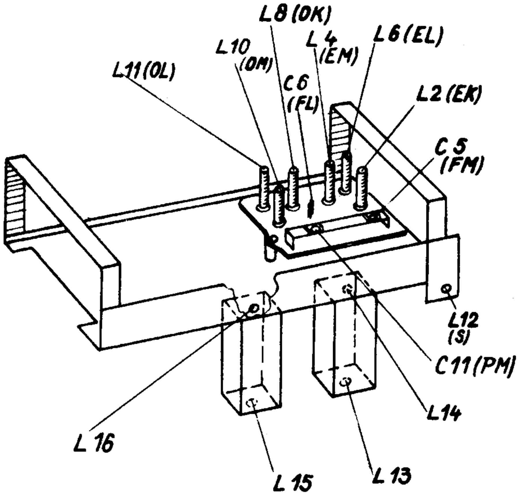
Zwischenfrequenz: 468 kHz L 16, L 15, L 14, L 13
