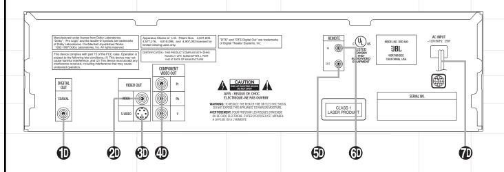
**©** Coaxial Digital Output: Connect this jack to the coaxial digital input of an A/V receiver or surround processor for Dolby Digital, DTS or PCM audio playback.
