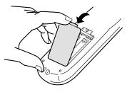
2 Place the two accompanying R6P(SUM-3)/ AA(15F) batteries in the remote control making sure to match the battery polarities with the markings ("+"/"-") inside the compartment.
