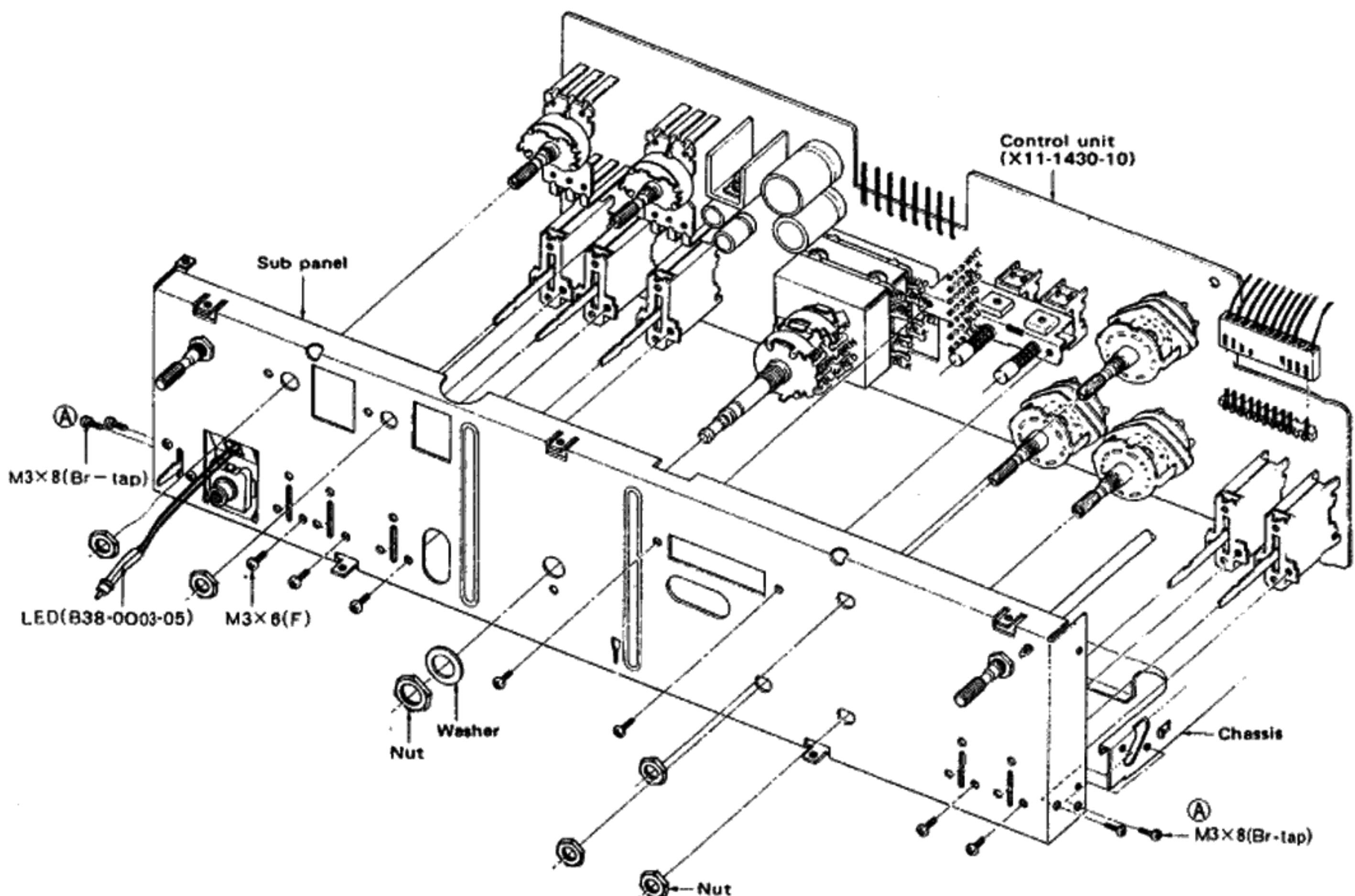
**< Disassembly of The Control Unit >**
