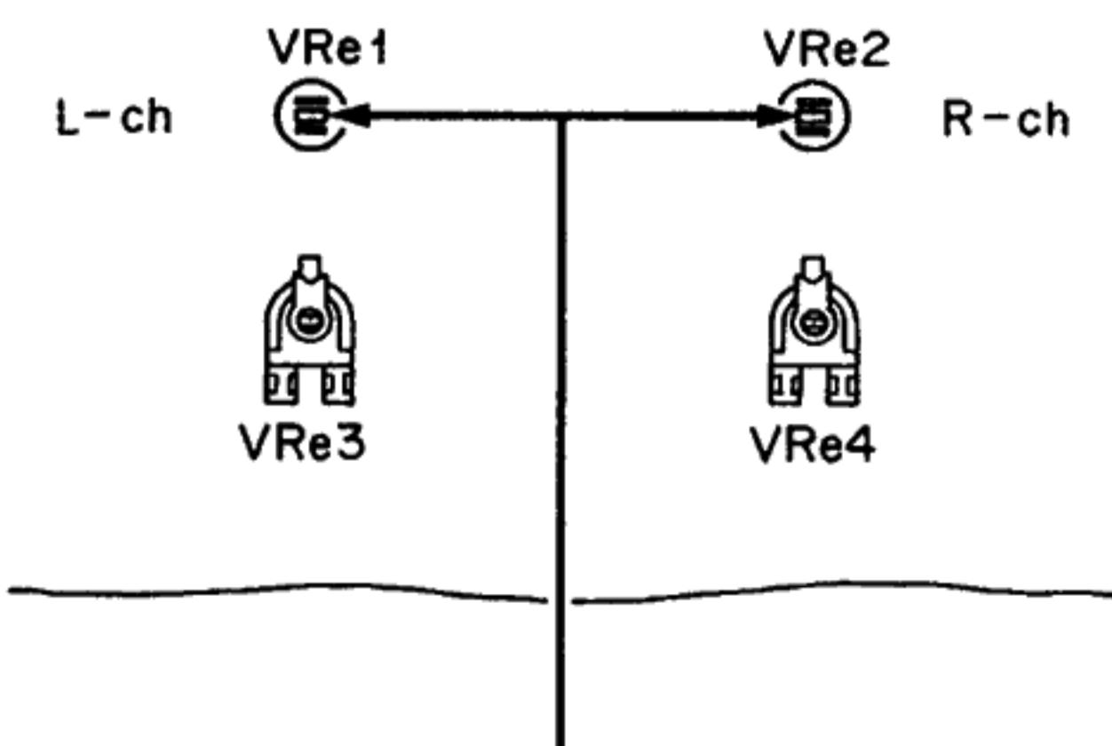
Turn the pc trimmer potentiometer VRe1 or 2 until the meter indicates OV
