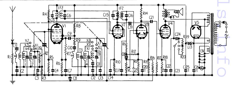
The K.B. 808 is a straightforward A.C. superhet and the components are well placed from a service point of view on a roomy chassis. The switch contact connections for the different bands are given in the text.
