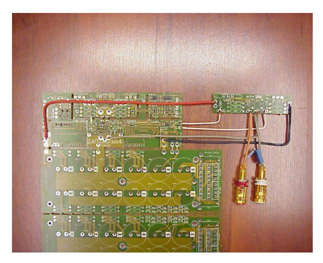
If You are using ext. Boards in a 78 or 118 Watt version, to drive a separate bass output ( the normal thing to do) You should connect a Zobel Network of a 100 nF / 400 V capacitor and a  $^2$ , Ohms 1 W resistor from Power Gnd to Output on the bass output ( as shown ). If You do not do this, using the one output with the other unconnected may cause oscillation, dangerous to the amplifiers health.
