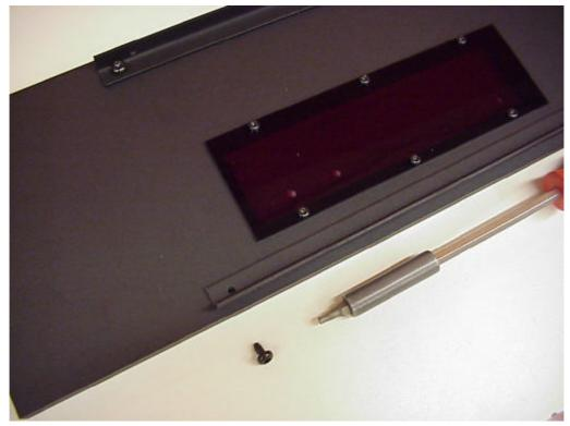
Use screw no. 2 for the brackets, and no. 4 for the front glass, be careful not to overtighten the front glass screws. A 'squeek' will sound when they are fastened properly. Fasten the front panel to the bottom plate using screws type 1.
