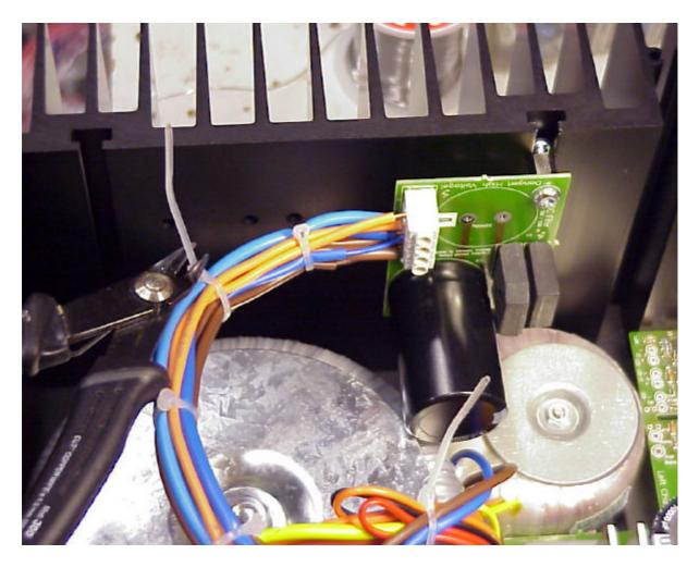
Fasten the DC filter to a heatsink as shown, it should be very secure, and the capoacitor must NOT be able to touch any cabinet part, when You put the lid on the case. You can tighten the spacer by holding the screw in the groove with a screwdriver while turning the spacer with a wrench. Then at last You tighten the screw holding the filter PCB.
