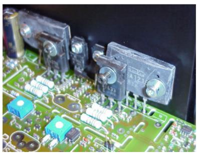
Screw on the output transistors, drivers and predrivers, so the distance from the PCB underside to the
