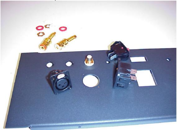
All holes are made to fit to the terminals, use screw no. 4 for the XLR receptors. The PUSH button should go upwards.
