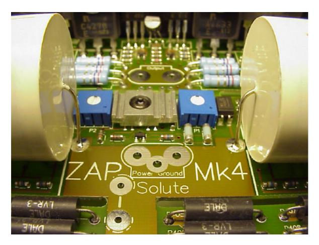
Now mount the input / output wiring, and switch wires.
