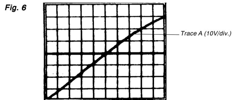
edge slopes: both must be 10V/μS or more as shown in Fig 6.
