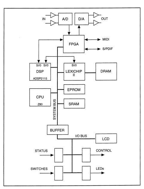
The Z80 handles the system software. The 2115 deals with signal routing and non-reverb DSP. The Lexichip performs the reverb. The FPGA performs most of the discrete logic, and includes an S/PDIF transceiver and MIDI UART. The EPROM holds the program information for the Z80 and the 2115, as well as configuration data for the FPGA. The SRAM holds variables for the Z80 and 2115, serves as a communication channel between the two processors, and provides a short audio buffer for the 2115.
