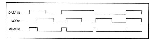
If the VCO leads the data in, this technique will not work, because the data stream doesn't have all of the edges the detector needs:
