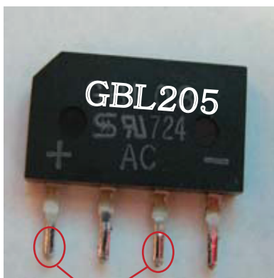
Check with ohm meter is short
