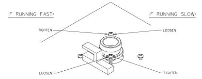
After adjustment, both screws should be in contact with motor topplate. Note: These screws should be snug only! Further tightening will simply bend the case of the motor, degrading the sound of the turntable and rendering proper speed adjustment difficult, if not impossible.
