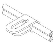
Slip the washer, P-clip, and associated nut onto the rear chassis bolt with the loop of the P-clip towards the rear of
