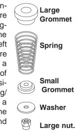
Each time you rotate a spring/grommet assembly, ensure that the entire assembly rotates during adjustment so that you do not introduce a twist in the spring. As you finish adjusting each spring, push up slightly and then release the washer on which the spring/grommet assembly rests. This will release any twist which may have been introduced into the spring.
