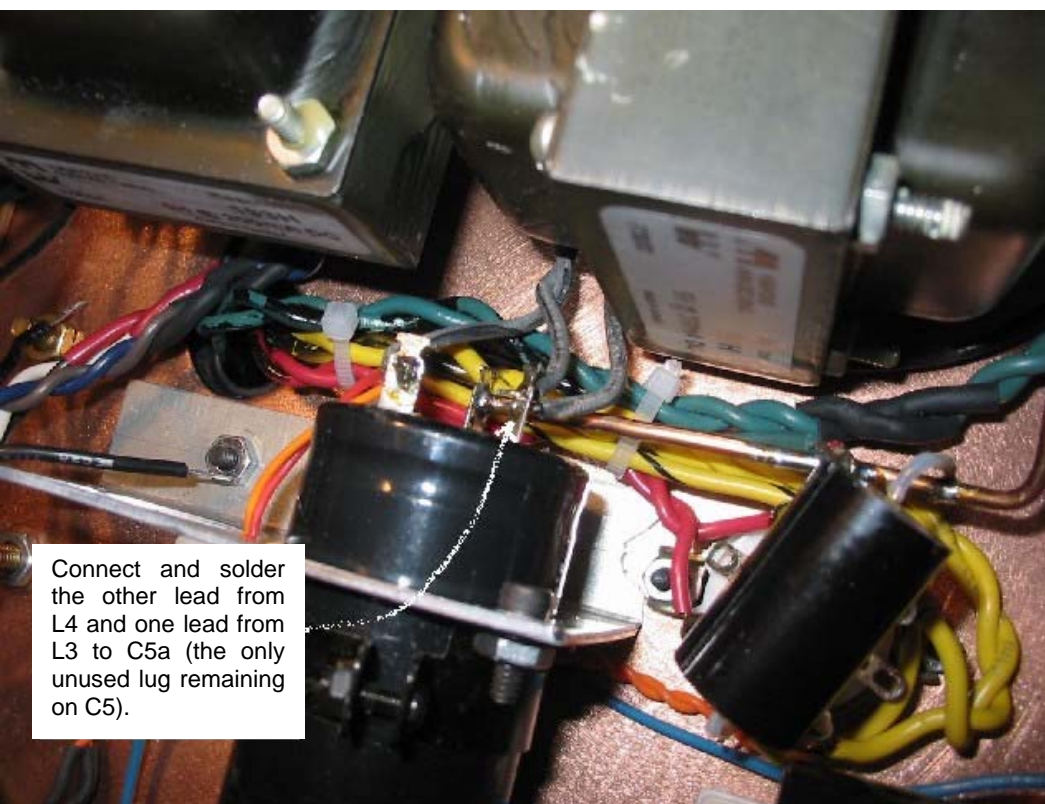
Figure 46. Wiring C 5a .
