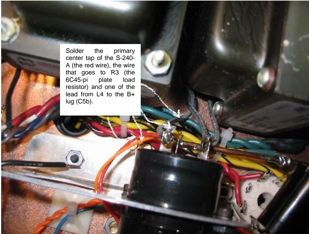
Figure 45. Wiring the B+ (C 5b ).
