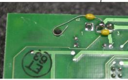
Add two 10kΩ, 1/8th Watt pull-up resistors across the Eprom devices: U11-pin 8 to U11-pin 5, and across U9-pin 8 to U9-pin 5. (Vcc and SDA).
