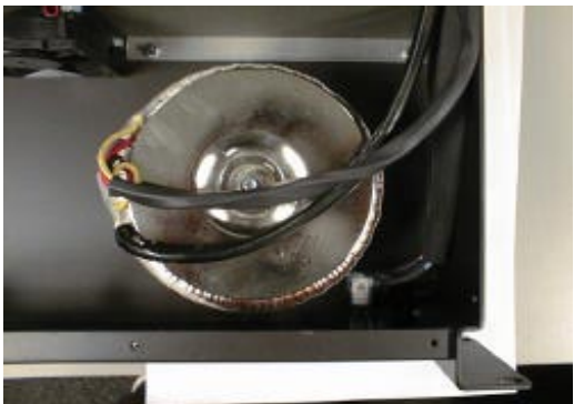
TRANSFORMER POSITION FOR 240V VERSION ONLY.
