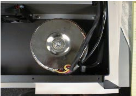
TRANSFORMER POSITION FOR 120V VERSION ONLY.
