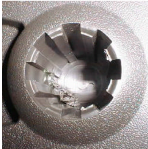
Plastic burrs from insert installation
