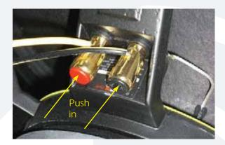
Remove cables from terminals simply by pushing down on terminal and pulling out cable.
