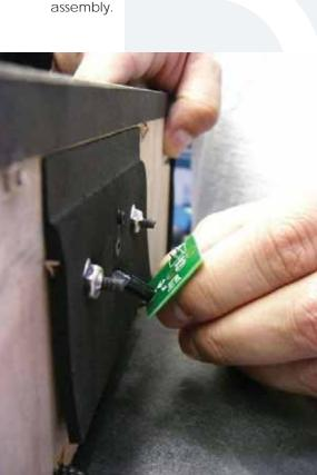
Carefully remove led PCB assembly from back side of front panel. A flathead screwdriver may aid in removal of led PCB assembly if it is sticking.
