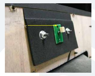
Use phillips head screwdriver to remove one screw from center of led PCB
