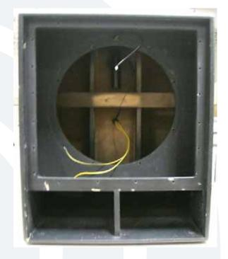
This is what it looks like with the front panel and woofer both removed. Place new woofer (part #0012184) where the old one was. Follow the same steps as above, but backwards 6 to 1, making sure to keep the led PCB assembly cable in front of woofer. Power up the SWA1801 and the new woofer should now be pumping out glorious lows. Awesome, you just replaced an 18" woofer!
