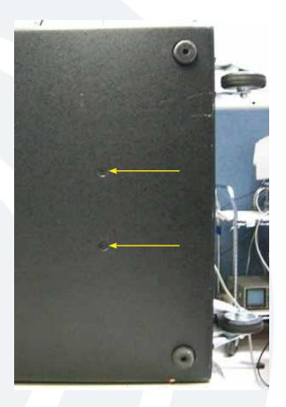
Last remaining two screws located on the bottom of the SWA1801.
