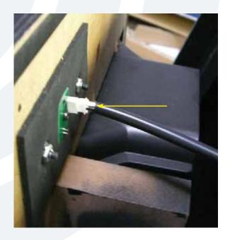
Carefully remove the cable attached to the led PCB assembly.
