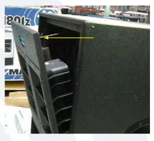
Carefully begin to remove the front panel. The wave guides are a great place to grip for stability and support. Do not fully remove front panel as the cable is still attached to the led PCB assembly.
