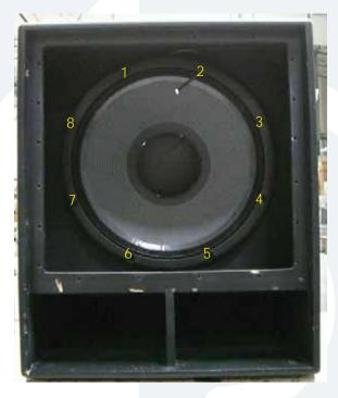
2 Eight screws need to be removed from the woofer using 5mm allen wrench.
