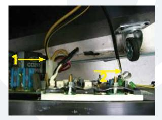
Two cables need to be removed from the amp assembly: (1) woofer cable (positive and negative cables on one connector) and (2) led PCB cable. Do not force cable removal or connection. Notice their placement, as well -- black wire of led PCB cable and yellow and black woofer cable are both closer towards the edge of the amp assembly.
