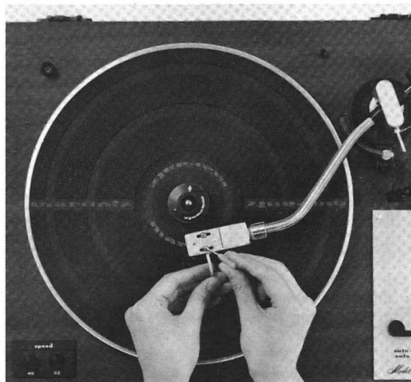
Figure 2. Stylus Overhang Adjustment
