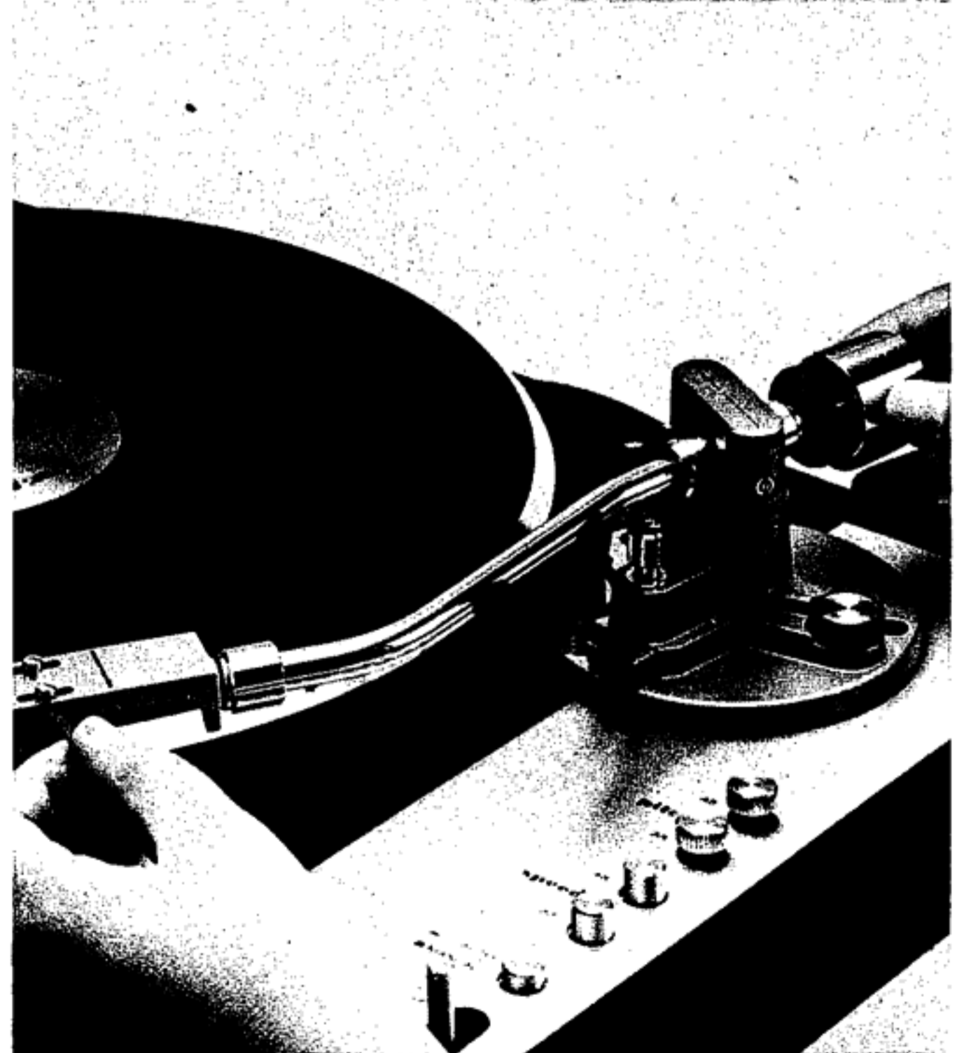
Figure 2. Tone Arm Balance Adjustment
