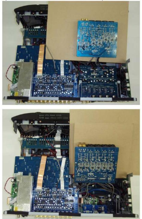
Put the Preout PWB on the insulator board.
