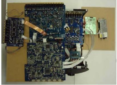
Change FFC: 17P 1.0mm (AV8003 A: Blue): CN71 (DSP) <--->CN72 (VIDEO) Change FFC: 13P 1.0mm (AV8003 B: Red): CN83 (DSP) <--->CN84 (HDMI) Change FFC: 15P 1.0mm (AV8003 C: Green): CN81 (DSP) <--->CN82 (HDMI)
