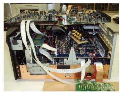
Put the Input PWB onto the insulator board and install the other PWB.
