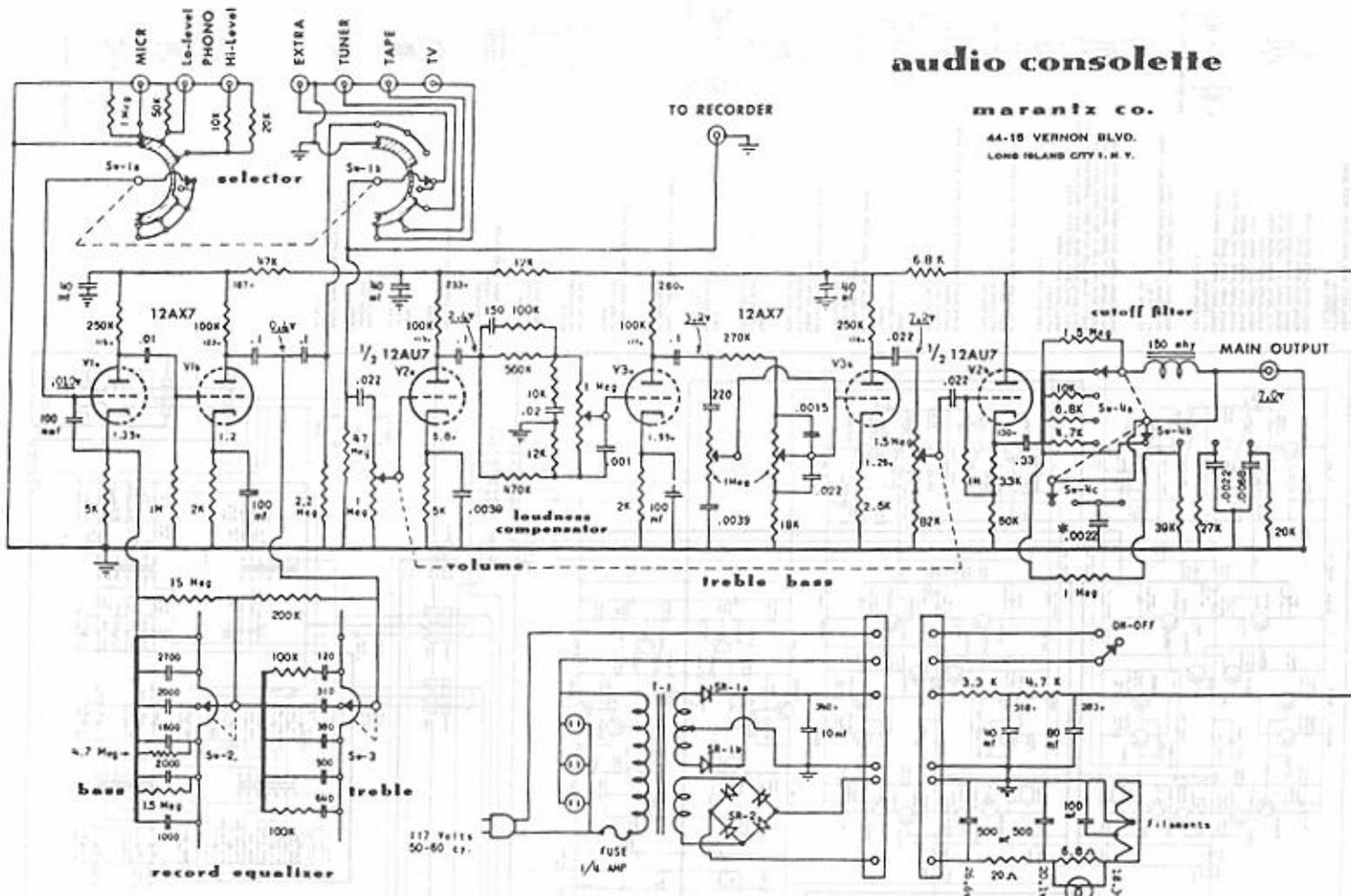
D. C. volts are approximate as measured with a V.T.V.M. after 30 min. warm up.
