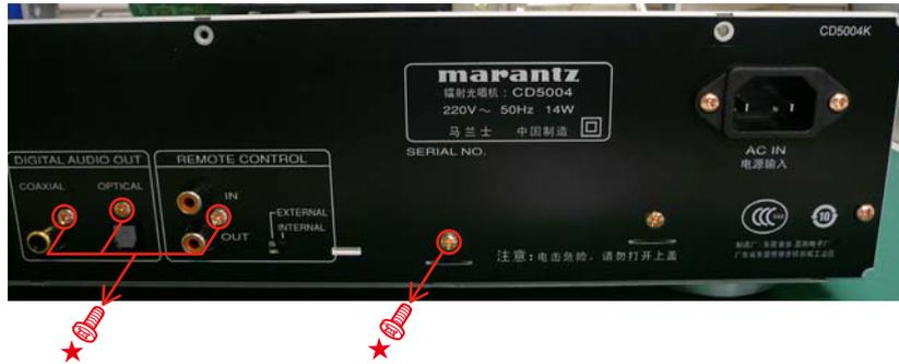
(2) Remove the screws. Disconnect the connectors wire and FFC Cable.
