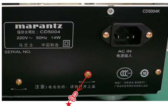
(2) Remove the screws. Disconnect the connector wires. Cut the wire clamp band.
