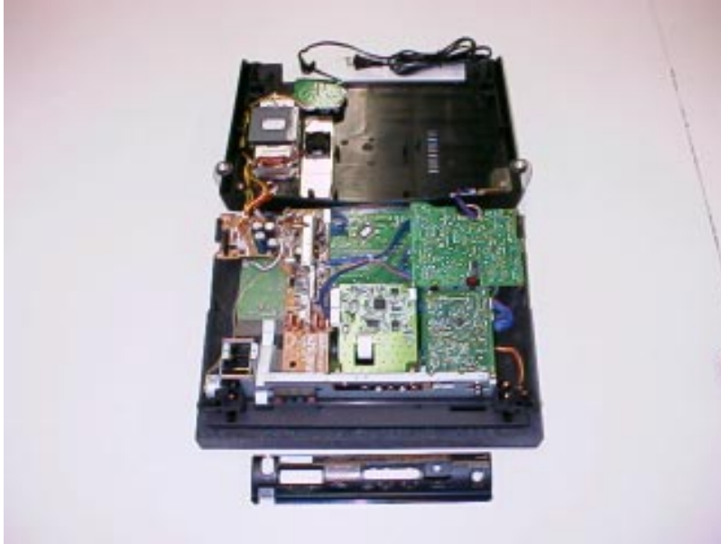
Fig.8 Taking the bottom case apart
