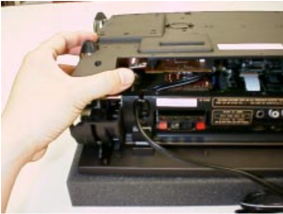
Fig.5 Lifting the bottom case
