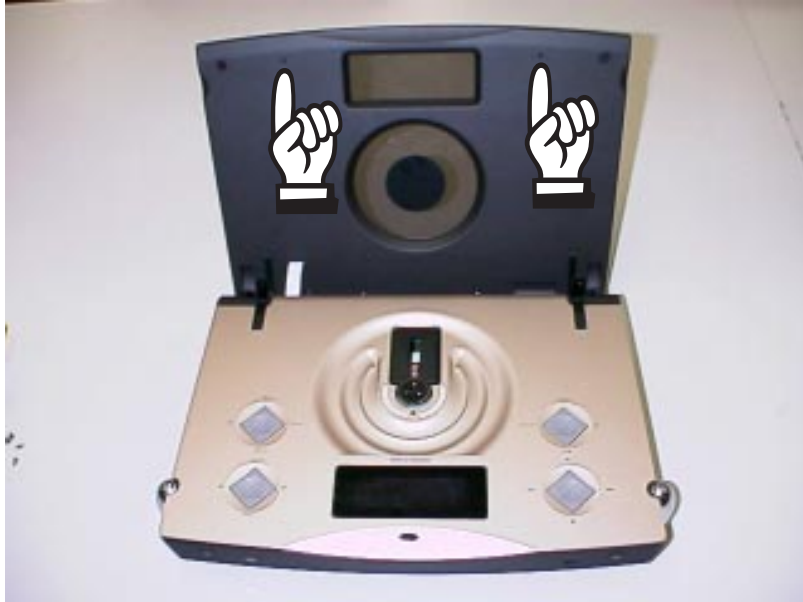
Fig.15 Positions of 2 screws on the top
