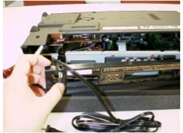
Fig.6 Removing the rear panel
