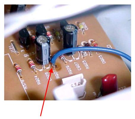
Solder the wire to the ground side lead of the R922 or R929
