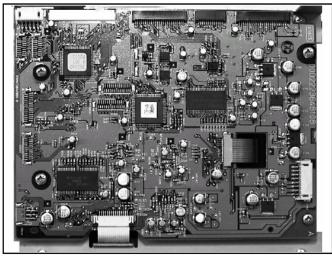
Mount POS.NO. R410 2.2K OHM (PART NO. 00D2472008926) onto the Super Audio CD PWB Module.
