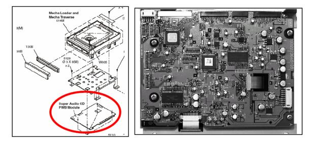
Mount POS.NO. R410 2.2K OHM (PART NO. 00D2472008926) onto the Super Audio CD PWB Module.
