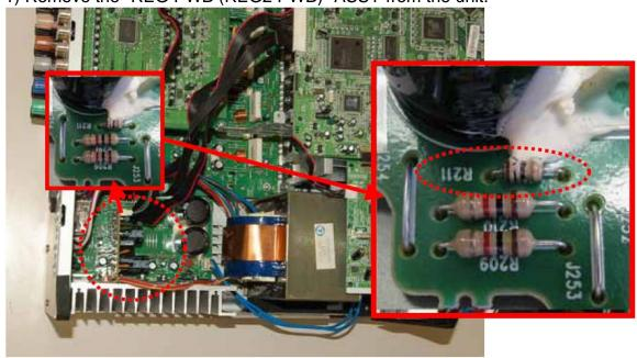
2) Short between both lands of pattern side of the R211 by thin copper wire. (Please do not cut the R211 10 ohms.)
