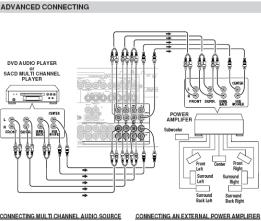
CONNECTING MULTI CHANNEL AUDIO SOURCE The 7.1CH INPUT jacks are for multichannel audio source such as a SACD multichannel player, DVD audio player or external decoder. If you use these jacks, switch on the 7.1CH INPUT and set the 7.1CH INPUT level by using the SETUP MAIN MENU. See page 28.
