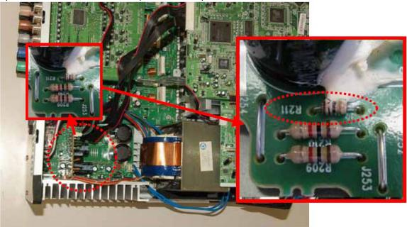
2) <u>Short between both lands of pattern side of the R211</u> by thin copper wire. (Please do not cut the R211 10 ohms.)
