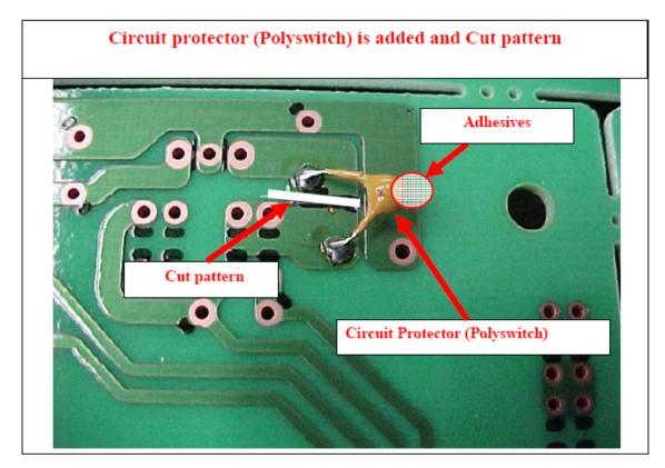
Adhesives: SC608LVZ (Sony Chemical Corp Self-extinguishing adhesive) or the equivalent.
