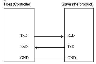
(Serial setting <RS232C basic>) Baud Rate : 9600bps
