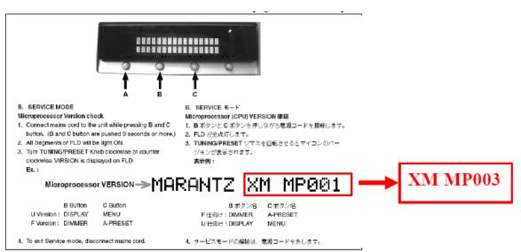
Before stating, check the firmware version. It can be confirmed through the "B.SERVICE MODE". Refer to the service manual ST7001/U1B on page 2 for the firmware procedure.
