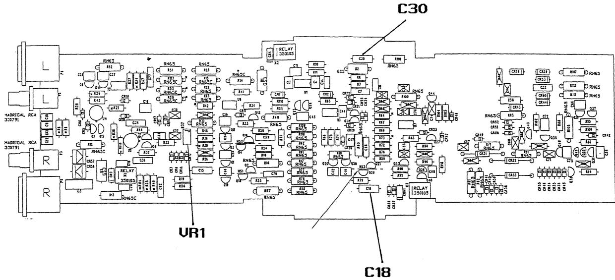
DC OFFSET ADJUSTMENT (after 2 hour warm up) Using DC voltage meter, measure across the (+) and (-) output terminals, and adjust VR1 for > 10mV.
