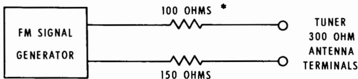
\* IF SIGNAL GENERATOR HAS OTHER THAN 50 OHM INTERNAL IMPEDANCE, USE A RESISTOR OF 150 OHMS, LESS INTERNAL GENERATOR IMPEDANCE.
