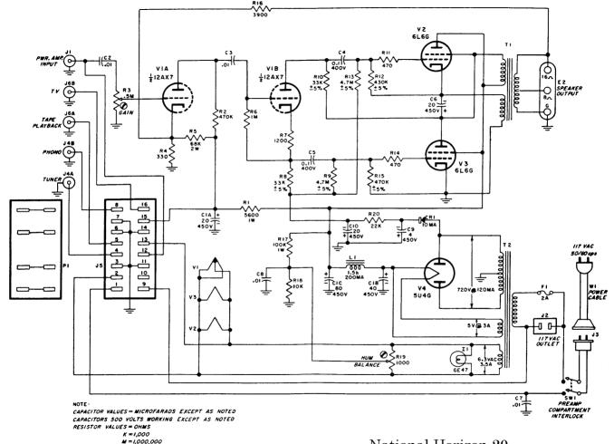
OMMIC VALUE OF FIXED RESISTORS ± 10% EXCEPT AS MOTED WATTAGE OF RESISTORS 1/2 WATT EXCEPT AS NOTED
