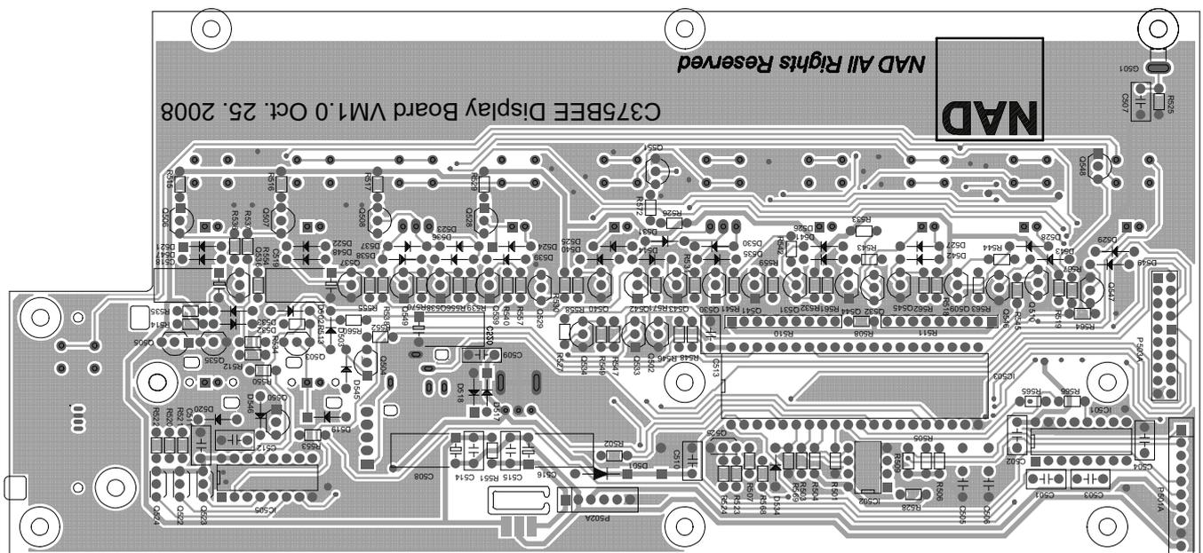
**PCB LAYOUT (Only replace Line In or Line Out modules, do not repair)**
