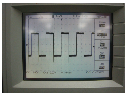
U1001 Pin 12 - Left/Right clock (PCM), 44.1kHz
