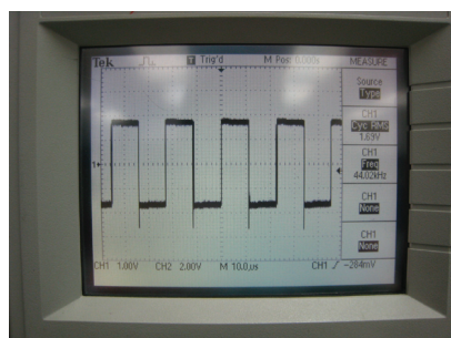
U1001 Pin 12 - Left/Right clock (PCM), 44.1kHz
