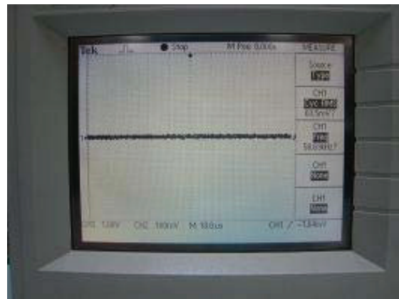
U9 Pin 4 –DAC_FLD (OSD Off), Idle
