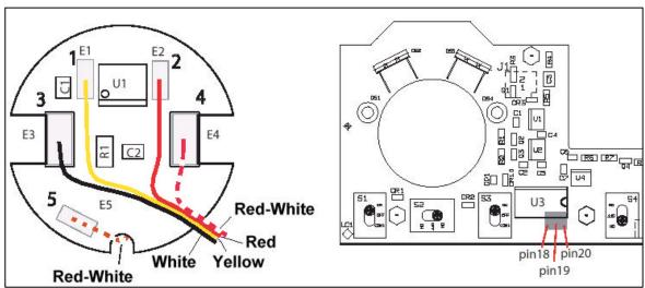
E4-Left modulometer (red needle) red-white (from previous connector with the red-white and the white wire).
