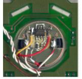
On the rear side of the red modulometer, solder the PCB. See picture. From the rear side, insert a red-white wire (60 mm) in the groove of the red modulometer. Solder the red-white wire on the PCB position E5. Solder the previously removed wiring on the added PCB (E3 is white, E4 is red-white)
