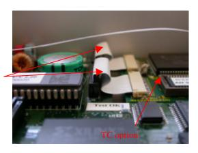
For the same reason, bend the ribbon cable between the box motherboard and the LF output PCB as close as possible to the LF output PCB.
