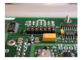
On the deck, remove the left 10 mm spacer this to install afterwards easily the ribbon cable.
