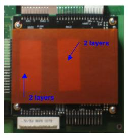
By using double-sided glue tape, add the insulator (0131 030 009) on the PC104 PCB
