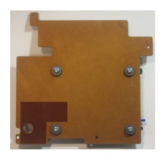
Install the internal HDD assembly on top of the deck mother board and fix it using the 3 nuts 5 mm "B", 1 screw "C" and 4 shims as shown.
