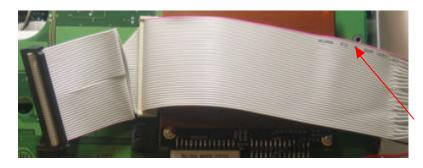
Install the new EDI ribbon cable (8131 405 000) by connecting it to the PC104 PCB. Verify that red wire from the ribbon cable is on top. Connect the power connector from the external HDD back to the deck motherboard. Connect the EDI connector to the external HDD. Put the deck motherboard back on the deck of the machine.
