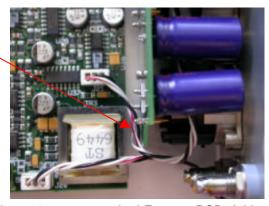
Reduce the pin size to maximum 1 mm versus the LF output PCB. Add some solder to remove any sharp edges.
