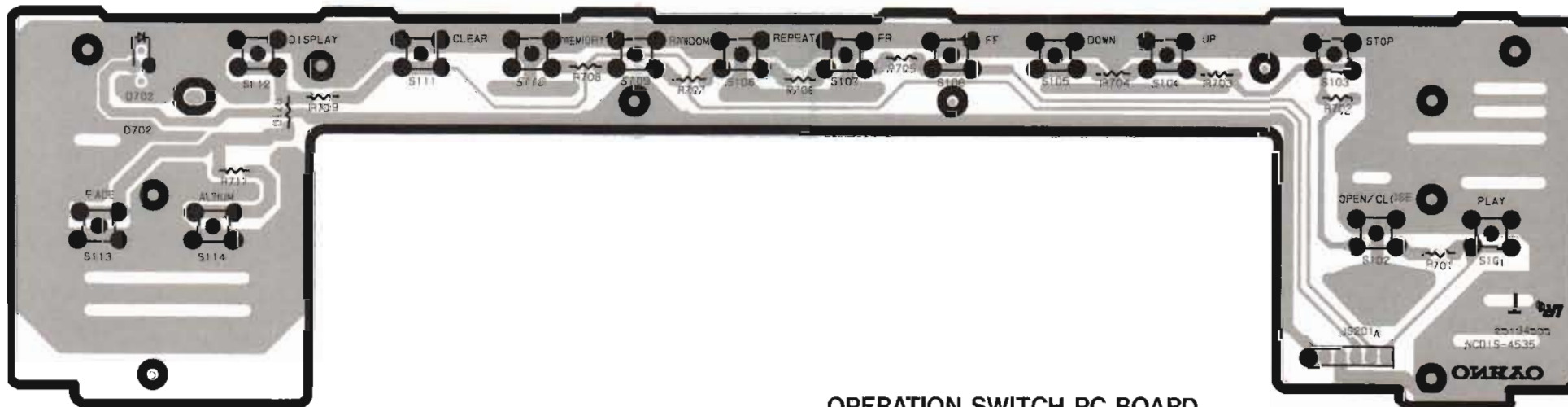
OPERATION SWITCH PC BOARD
