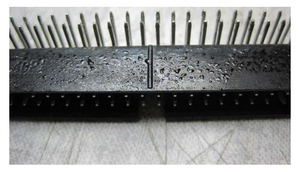
**Cause**: Insulation failure between pins of IDE connector(s) might cause erratic behavior of Microprocessor. Contact problem in IDE cable from display board to micro board.
