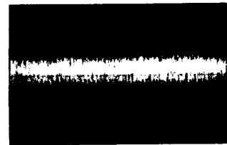
Tracking signal P108 pin 4 (HF) V: 20mV/div H: 0.5mS/div
