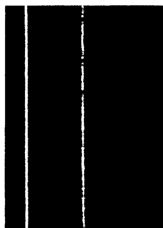
DATA (Microprocessor) Vertical : 2V/div. Horizontal : 0.5 ms/div. DC, Ground: Center
